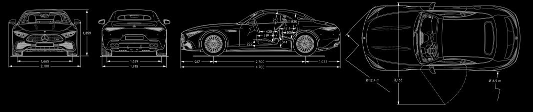
All measurements in millimetres. The dimensions shown are mean values and apply to standard-specification, unladen vehicles
