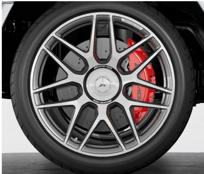
RG5 22" AMG forged wheels – cross-spoke design, painted titanium grey with a high-shine finish, 295/40 R22 tyres
