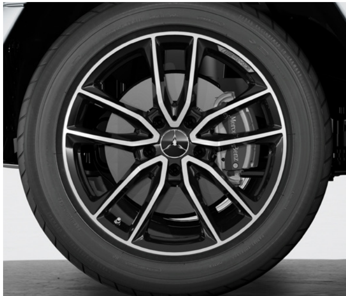
R16 20" AMG alloy wheels – 5-twin-spoke design, painted high-gloss black with a high-sheen finish, 275/50 R20 tyres
