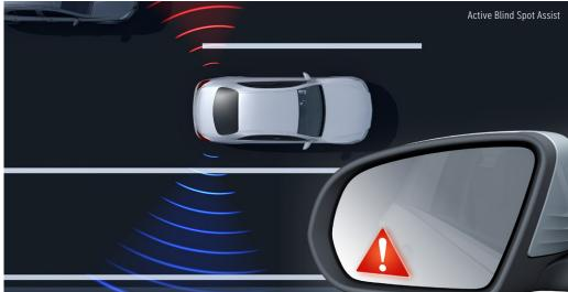
Active Blind Spot Assist can warn the driver of vehicles in the blind spot during a lane change
