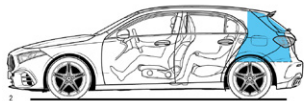
2 Open luggage compartment behind rear seat, loaded to roof, volume 435 litres (V 214-2)
