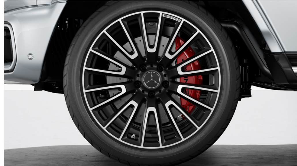
R20 22" AMG forged wheels - multi-spoke design, painted matt black with a high-shen finish, 295/40 R 22 tyres
