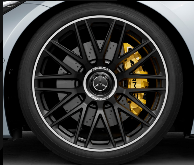
RWE 21" AMG forged wheels - 10-twin-spoke design, painted matt black with a high-shine rim flange, 295/30 (front) and 305/30 (rear) R21 tyres
