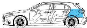
1 Open luggage compartment behind rear seat, loaded to upper edge of rear seat backrest, volume 355 litres (V 211-2)
