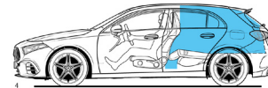
4 Open luggage compartment behind driver's seat, rear seat backrest folded, loaded to roof, volume 1,195 litres (V 214-1)
