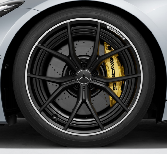
21" AMG forged wheels - 5-twin-spoke design, aerodynamically optimised, painted matt black with a high-sheen rim flange, 295/30 (front) and 305/30 (rear) R 21 tyres (code RWK)
