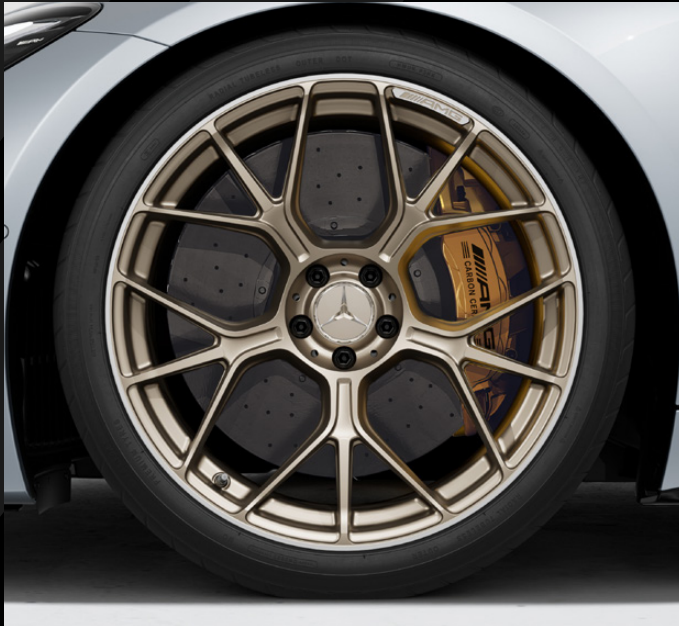
21" AMG forged wheels - cross-spoke design, MANUFAKTUR version painted matt techgold with a high-sheen rim flange, 295/30 (front) and 305/30 (rear) R 21 tyres (code RWM)
