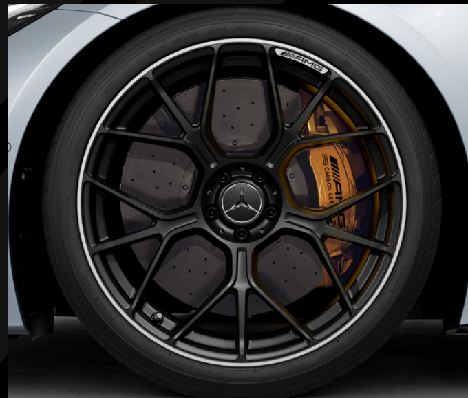
21" AMG forged wheels – cross-spoke design, painted matt black with a high-shine rim flange, 295/30 (front) and 305/30 (rear) R21 tyres (code RWL)
