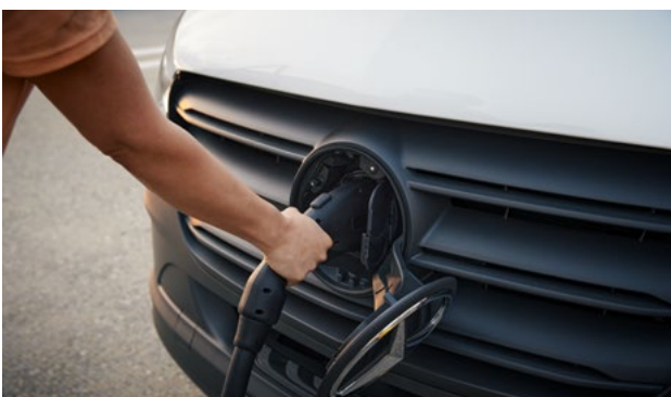
CCS rapid charging port, 115kW max. capacity.
