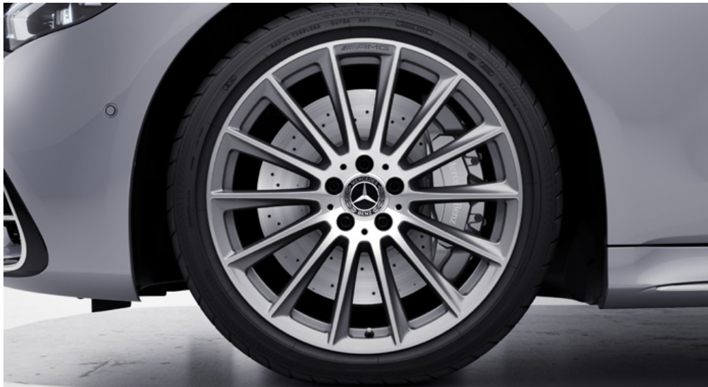
RVQ 20" AMG alloy wheels – multi-spoke design, painted himalaya grey with a high-shine finish, 255/40 R20 tyres
